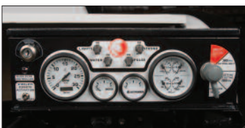
Marine-grade gauges and Spartan's exclusive Dial-A-Pressure PSI settings simplify operation.
